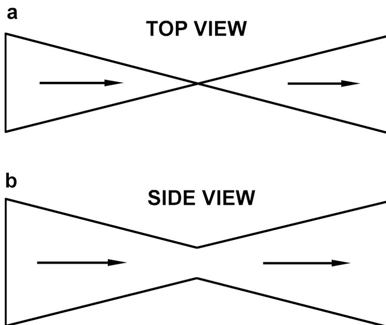
**Fig. 2.24.** Typical sample beam in a dispersive instrument with a slit image as seen from above (a) and as seen from the side (b).
